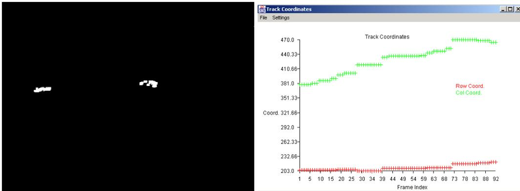
Figure 3: Example of analysis at the event level. Top row shows two frames from a video sequence with two moving vehicles entering a parking lot. Bottom row shows detected vehicles as white blobs (left) and the plot of tracked pixel coordinates of the white pickup truck (the vehicle on the right side) as a function of frame index (time).
