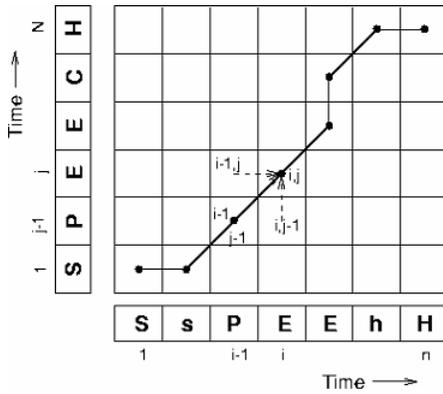
Figure 3 : Illustration of DTW algorithm used to compare two instances of the word "speech". The picture shows the shortest global path from beginning to end, as well as the calculation of error at coordinates (i, j).
