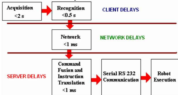
Figure 6: Delays occurring between the time a command is given and executed by robot
