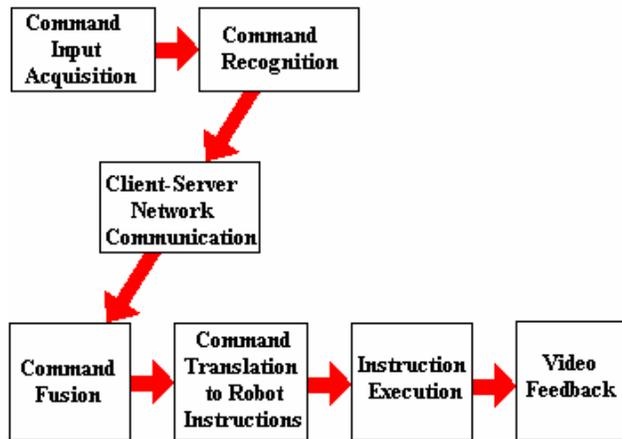
Figure 2: Robot control system flow. Command acquisition and recognition are described in Section 2. Network architecture is outlined in Section 3. Command fusion, instruction translation and execution, followed by video feedback are overviewed in Section 4.
