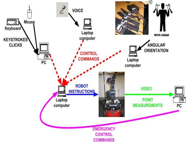
Figure 1: An overview of a system for remote robot control using sound, gesture and human-computer interface inputs.
