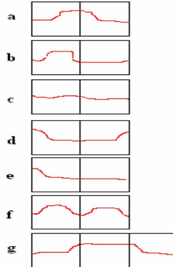
Figure 5: Possible cases of voice signals within the one second segments. They are: (a) one command spread across 2 seconds; (b) one command in one second and silence in the next; (c) silence; (d) end of command in first second and start of another command in 2nd second, (e) end of command, (f) 2 quick commands in succession, and (g) command spread across 3 segments.
